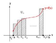
Let  $\Delta$  denote the quantity  $\frac{b-a}{n}$ , i.e. the width of a small strip. Then  $c_k = a + k\Delta$  and the shaded area, which we call  $U_n$ , is given by
